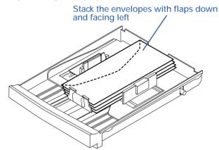
**WARNING!** Do not use envelopes that have fasteners, snaps, or windows. Also, do not use envelopes that seal with peel-off strips or pressure-sensitive adhesives. Printing on such envelopes can damage the printer.
